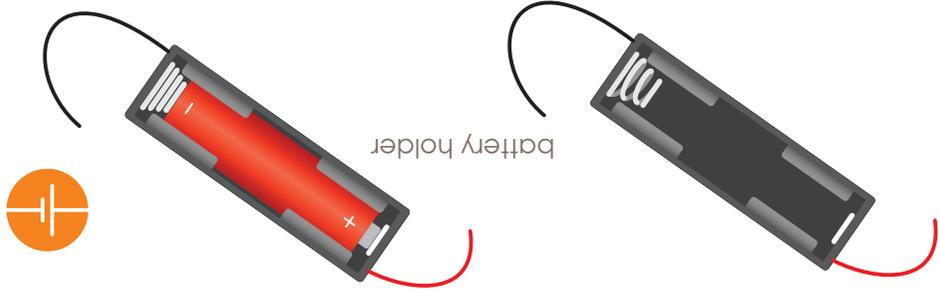
To make connection to your battery, press the negative (flat) end of the battery against the spring and push down until the battery fits snugly inside the battery case as shown below.
