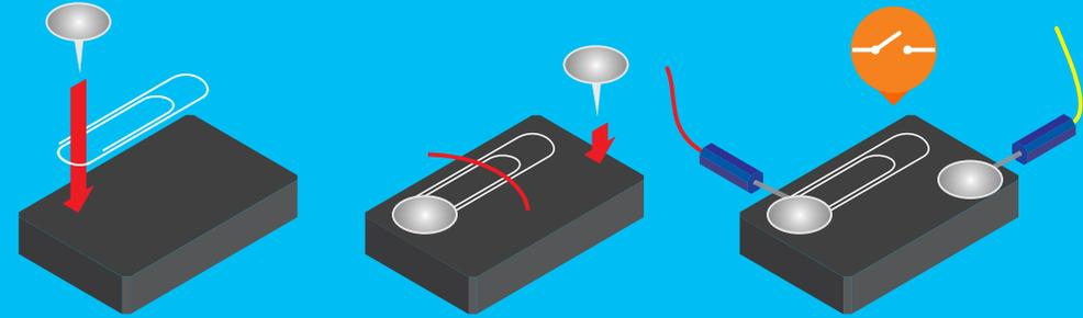
Connect the switch into your circuit. The buzzer should make a sound when close the switch and stop when the switch is
